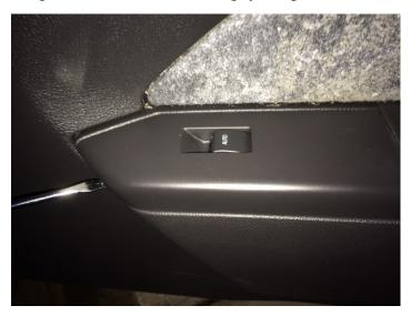
5. The last piece of removable plastic is the square-shaped piece of plastic in the middle of the armrest behind the handle. Pry it up from the top, this may require some forceful pulling, make sure you don't scratch it. Remove the T30 screw below this panel.
