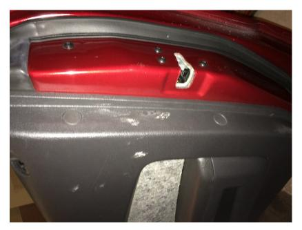
9. Now, once you're sure all the screws are off, you should be able to lift the door off the frame. There is one additional electrical plug you must disconnect from the lock button on the door handle. The door handle is also held in place by, basically, a bicycle-brake-style assembly. Use a pair of needle-nose pliers to squeeze
