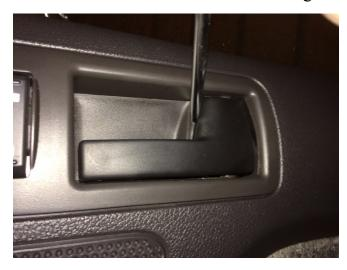
3. Remove the lock pin cover at the far end of the door by prying it carefully upwards from the bottom using a small phillips flathead screwdriver.
