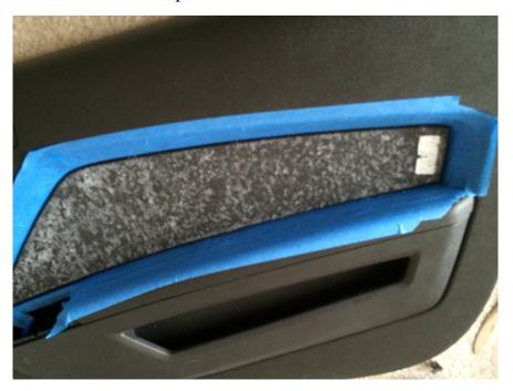
15. The RedlineGoods inserts came with a bit of excess fabric. That is on purpose, it's better to cut a tad too wide, than too narrow. © Trim small strips off if necessary, so that the glue would be able to stick to the leather properly.
