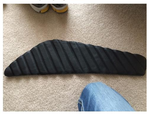
Used DAP Weldwood or similar spray adhesive in order to attach the inserts to the door. It is a high-quality, high strength long hang time adhesive that is commonly used for automotive upholstery. It can be found at many stores such as Menard's or Home Depot. Spray the back side of the door panel insert, making especially sure to get the edges.
