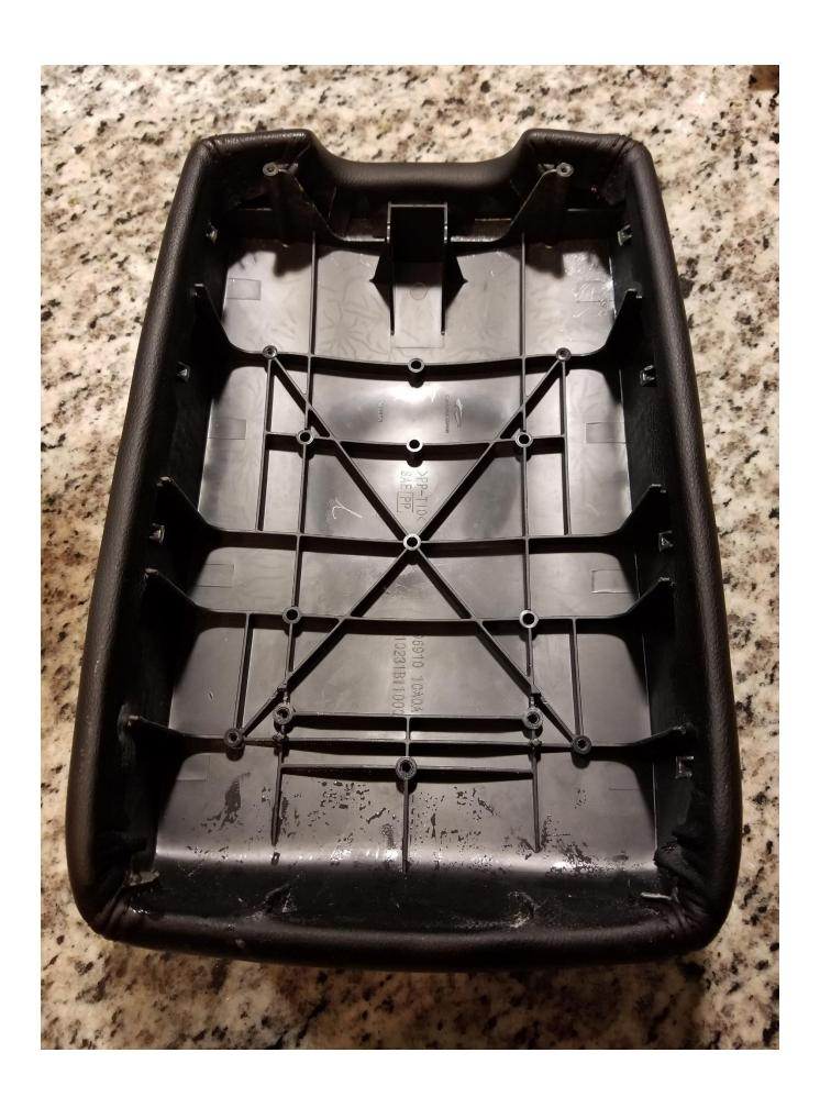
Assemble in the reverse order of removal – reinsert the 3 screws with flex extension:
