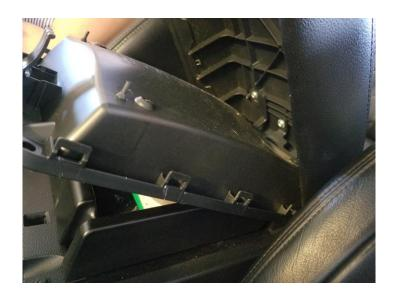
Most complicated part. TO remove 3 screws in the back (it hard to remove without flexible extension) or you can use bit + vise grip:
