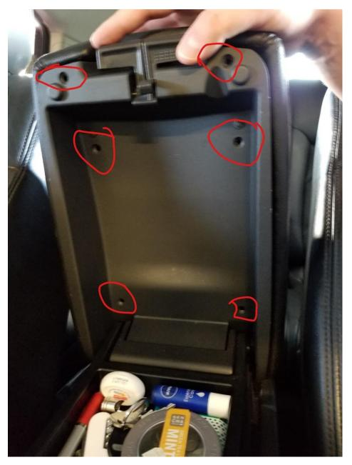
Pry off with clip removal tool (you can use knife or plastic card) to get the outer layer off:
