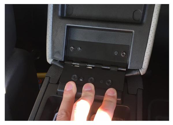
Remove these three screws and remove the lid. Separate the top and bottom halves of the armrest.
