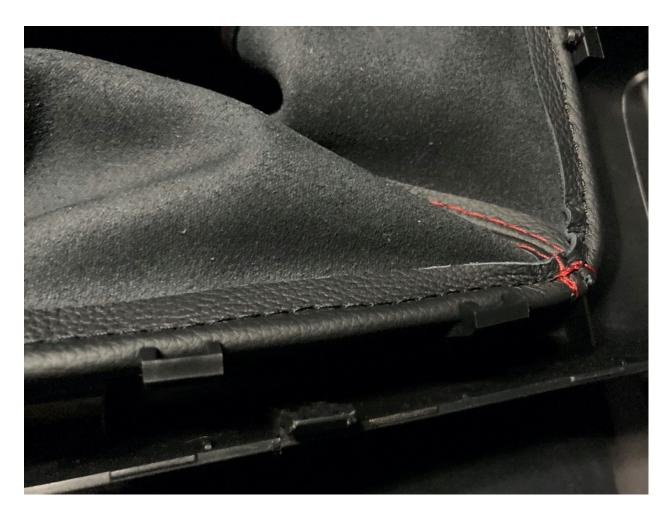
8. THE SHIFT BOOT CONSOLE JUST POPS BACK IN TO PLACE, PUSHING ON EACH OF THE CORNERS CAREFULLY.
