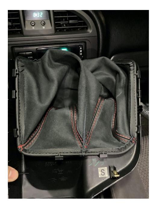
6. YOUR OLD SHIFT BOOT WILL BE SECURED ONTO A FEW OF THE NIPPLES PICTURED BELOW WITH SOME PUSH ON WASHERS HOLDING IT IN PLACE. GRAB A PAIR OF NEEDLE NOSE PLIERS AND CAREFULLY PULL THE WASHERS OFF. YOU WON'T HAVE TO REUSE THEM WITH THE NEW BOOT.
