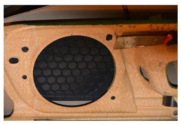
If you're replacing the lower front door vinyl, you have to remove the large plastic piece from the insert card. There are 14 fasteners holding the piece. Remove those similarly to speaker grill.
