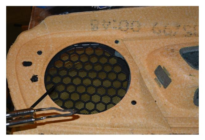
If you use a new speaker grill, simply melt the tips onto panel. If you're able to recovery old grill, use some zip ties to melt over posts and fasten.
