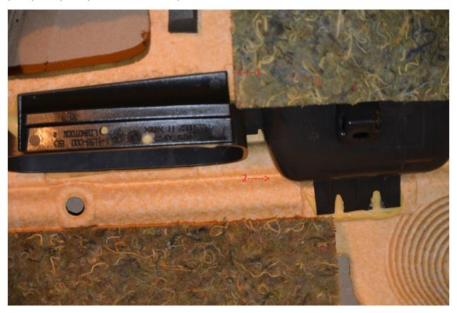
On the front doors, the speaker grills are fastened in place by the melted tips of the speaker grill posts. The fasteners can easily be broken off by prying around with a putty knife or similar tool. Once removed, the speaker grill can easily be removed without any resistance. The speaker grills break very easily, so be careful! Remove remaining switches from doors.
