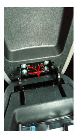
Step 2: Remove bottom of console lid by removing 4 screws
