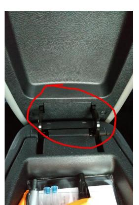
Reinstall console lid bracket with 4 silver replace the cover.
