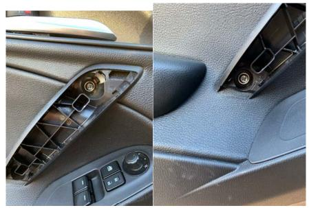
1. Remove these screws and from here using the pry tools insert between the card and the metal door in-between the weather stripping and pull the panel towards you. Once all the clips are loose pull up on the door panel and guide the door handle out the back and undo the plugs for the window switch module and in the case of the driver side, the mirror adjustment module. Once removed it should look like this:
