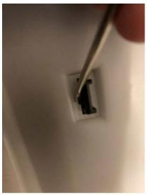
The arm rest should pop off with little to no hassle. Remove and set to the side.
