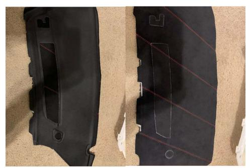
Cut the traced holes out.
