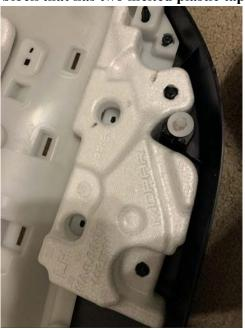
Gently lift on that part, the plastic tabs should just slide out and take little to no foam with it as in my case, but if there is an issue where the plastic tabs break, super glue can be used to re-attach.
