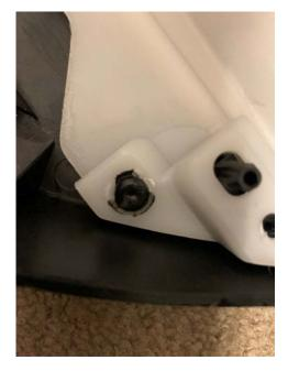
6. Next, once those tabs are broken or removed, the final disassembly part is the electronic switches for windows, doors, and/or mirror controls, there is 1 side of plastic tables that must be CAREFULLY pushed in as seen in the picture below:
