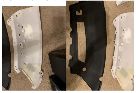
(Tip: As can be seen in the photos, FCA/Mazda put a large amount of adhesive towards the front of the panel, so if you can try to find an adhesive remover to remove a large amount of this extra adhesive. Once that is done clean and dry the area because the adhesive remover will cause an issue when gluing on the door card.)
