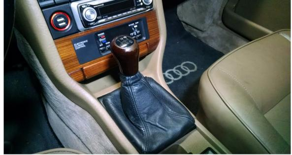
Go ahead and remove the shift knob now, which just unscrews from the shaft. Next remove the carpeted side panels on either side of the shifter. There is a small carpeted tab towards the front of the panel that you lift up to expose the Phillips screw underneath:
