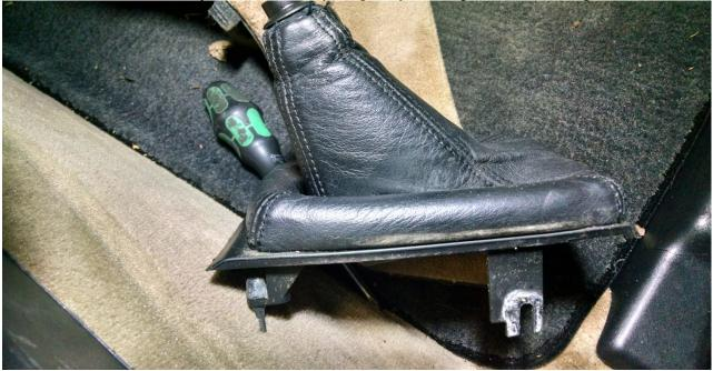
Flip the assembly over to reveal the four small screws in each corner.
