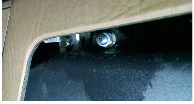
This provides access to the shift boot bracket screws which then get removed from each side:
