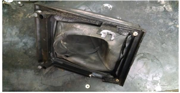
Once removed, the two lower sections come apart as well as the threaded shift knob collar and the inner rubber boot.
