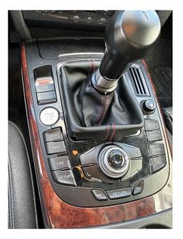
Cut the metal clip or zip tie retaining the old shift boot. If your car has the factory boot and knob and has never been altered, it will be a metal clip. Most aftermarket solutions require a zip tie.
