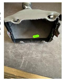
The shift knob and boot assembly can now be reinstalled. This can be done by installing the knob onto the shifter shaft and then pressing the frame into place. The assembly can also be installed by installing the frame first and then pressing the knob onto the shifter shaft.
