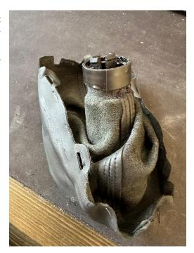
The plastic ring holds the shifter boot to the knob. This needs to be carefully pried up so that the boot can be removed. If you wish to reuse the factory shifter knob, be careful not to break this part.
