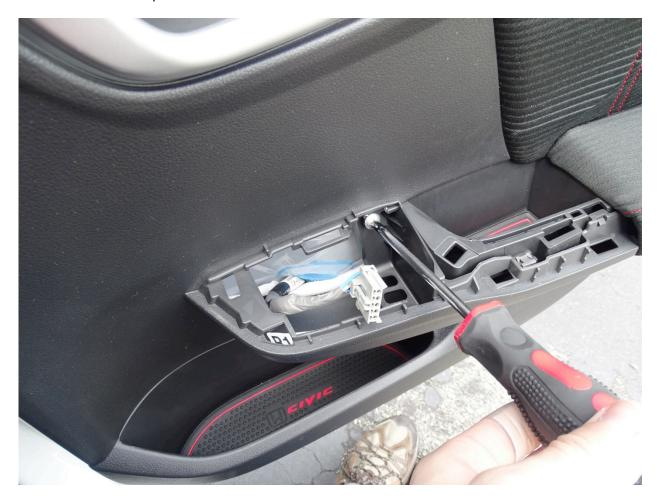
There is a little gap at the bottom of the door in the center to use as starting point when praying apart the snap clips. Just work your way around the clips and lift vertically once they are all no longer secured.
