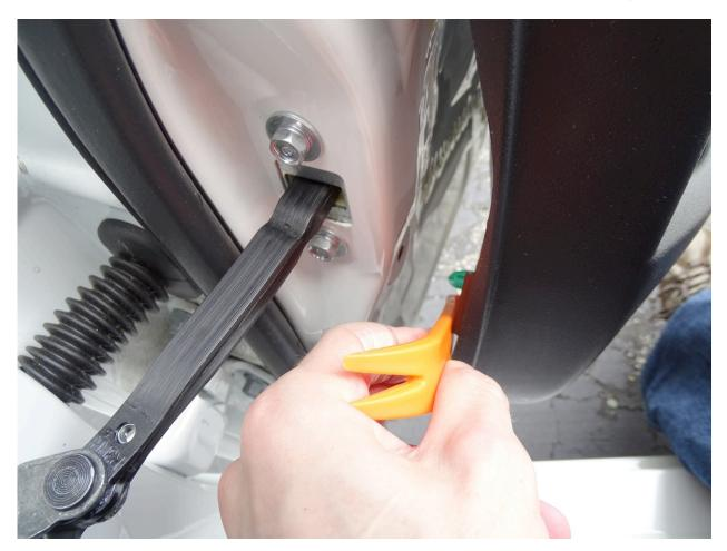
You'll need to break the plastic welds to get the inserts out. I found this to be easier using a heat gun to soften up the plastic making sure to not melt the door and using a dremel and box cutter to carefully cut away the plastic. The small flat head screwdriver was helpful as well you poke through the last bit if it didn't come apart. This is the rear passenger door.
