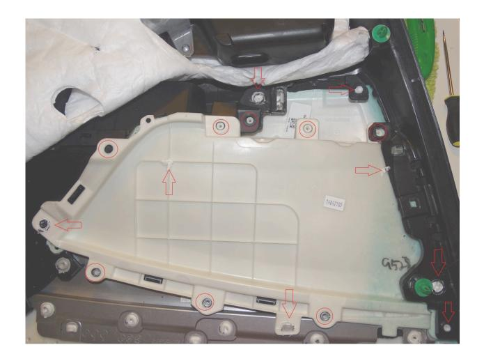
Once the inserts are out you'll need to carefully remove the stock fabric. Test fit the new fabric/leather as you may need to trim it slightly. I found the foam backing around the edges to be a bit thick and needed to trim it to fit properly. It'll depend on what options you choose so you may not need to do this step.
