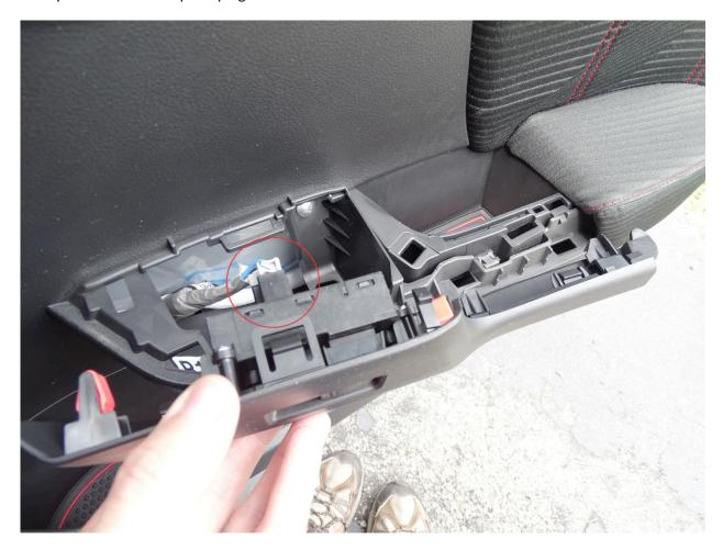
Next unscrew the Philips head screw and set that off to the side as well.
