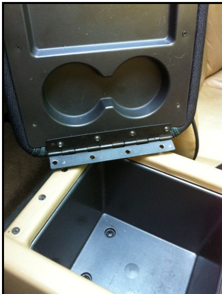
Figure 4 – armrest ready for re-installation
