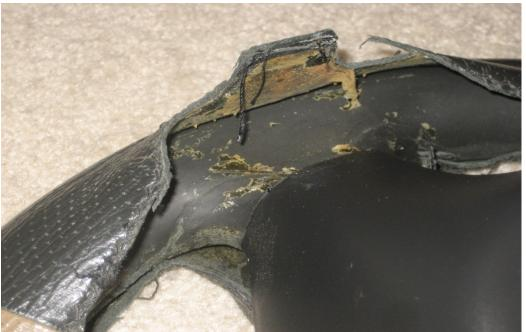
Once the skin is off, you will now need to remove the dark colored plastic backing that is on the back of the wheel, it is held on by four Philips screws
