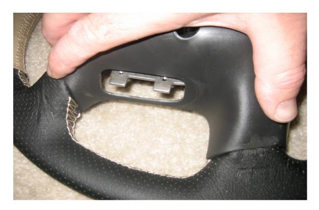
It is a tight fit, but you want the leather to be under the cover as it will give it a more finished look. Finally once you screw the backing piece on, then you are ready to put back on the cruise and radio controls if equipped. You now have a nice looking wheel.
