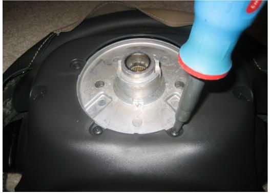
After removing the four screws, you need to remove the cruise control and radio controls from the wheel if yours is so equipped. Doing this requires the same size Phillips screws to be removed.
