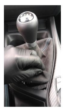
2. Once the shift boot trim is free of the center console, firmly grasp the shift knob and pull upward. It will take a lot of force to pull the shift knob free but it will eventually pull off along with the shift boot and shift boot trim.
