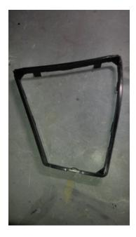
5. Test fit the new shift boot on the plastic shift boot frame. Look for any areas that may need trimming after attaching the frame to the shift boot.
