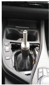
4. Use needle nose pliers or other tool to remove staples that hold OEM shift boot to the shift boot trim. Work carefully and take your time not to damage the trim, it is prone to cracking. After removing the staples carefully pull the shift boot off of the shift boot trim piece. It is held on by some adhesive but will come off relatively easily. A heat gun can make this step a little easier. You will be left with the plain plastic frame when you are done.
