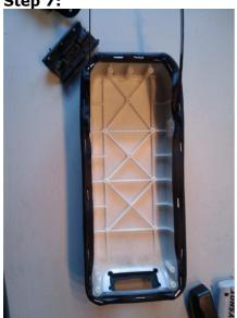
The most convenient way to do this is if you have a stapling machine. Pull the leather over the armrest firmly and every few centimeters, secure the leather by stapling it to the original vinyl cover.
