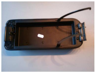
If you don't have a stapling machine, you now have to put the three plastic parts (taken off in step 2) back into place and screw them back, but you need to make sure that you cram the leather in between the armrest shell and the plastic part to ensure a nice end result. This is where a small flathead screwdriver might come in handy to push the leather in, but be sure not to damage the leather with the screwdriver!
