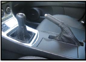
10. To install e-brake boot, simply pull over end and into place.
