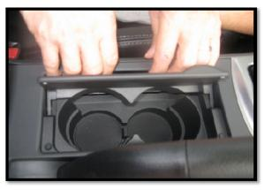
1. Remove shift knob by turning anticlockwise, set aside. Open cup holder in center console and place fingers on edge along drivers seat.
