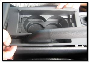
3. After drivers side is loose, gently pull straight up on passenger side edge of cup holder. Remove entire assembly and set aside.
