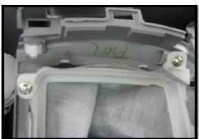
7. On the underside, remove two screws toward rear of shift boor surround and remove plastic retainer.
