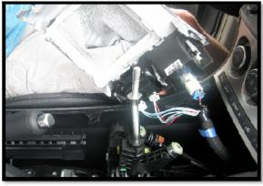
6. Remove entire shift surround and set aside being careful not to scratch any of the plastic surfaces. If necessary, unclip wires attached to seat heaters and accessory socket.
