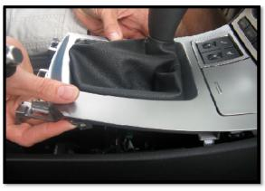
5. After rear clips are loose, move forward and loosen the middle and front clips by gently pulling straight upward.
