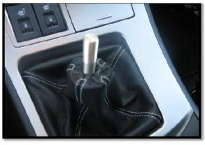
9. Reuse the top trim piece from the old boot and install it on the new one as well. Replace shift knob by screwing into place.
