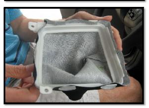
8. Remove retainer from shift boot surround and then remove shift boot from retainer. Install new shift boot and reinstall in reverse order.
