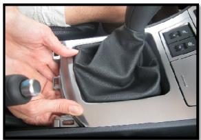
4. Place fingers under rear edge of plastic shift boot surround and gently lift upward loosening clips at rear.
