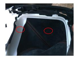
Install the plastic ring you separated from the OEM shift boot on your shift lever.
