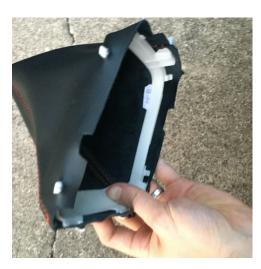
Re-attach the shift boot/retaining ring to the shifter console trim. The teeth (circled here) need to go in first. Then you can re-install the two screws.
