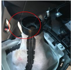
Install your new RedlineGoods shift boot on the plastic retaining ring.
