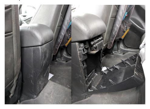
After removing the rear cover of the center console there are 4 phillips screws that you need to remove in order to separate the center console lid. 2 screws are located on each side of the center console.
