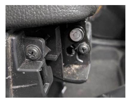
After removing the 4 phillips screws the center console armrest should just lift off.
