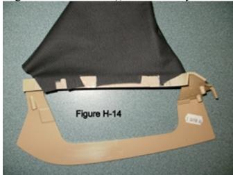
Do this by applying the glue quickly to the inside edge of the leather boot, a few inches at a time, and affixing it to plastic cover. By the way, it seems to work best to line up the deepest point of the two notches in the boot with the edge of the plastic cover.
