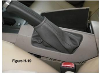
Work the top of the boot into the narrow channel just below the bottom of the handle, and make sure it is seated properly.
