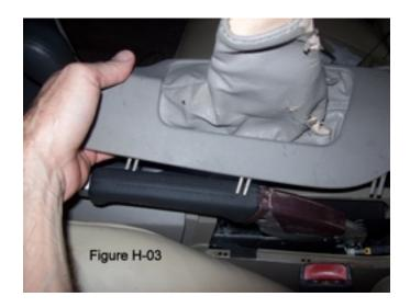
(3) Now, turn the boot assembly over. You will see the inner and out boot covers. The outer cover is grey, while the inner cover is tan.
