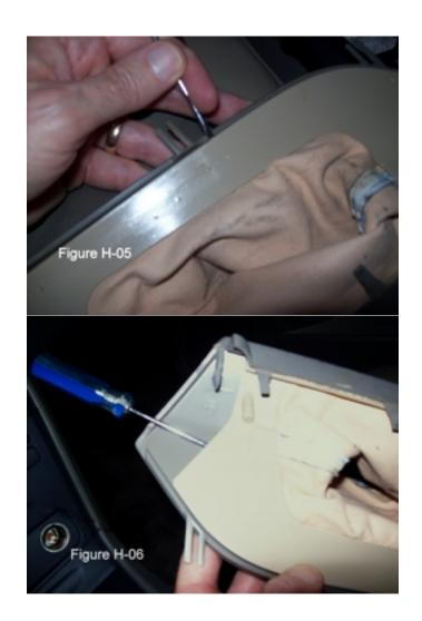
(4) Pry out the staples which hold the boot to the inner cover.
