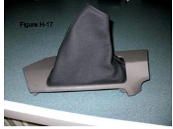
(9) Before you install the boot there is one more step: Take a pair of scissors and trim off any excess material (especially at the seams) from the inside of the opening of the boot. Since the new leather boot is thicker than the old imitation leather boot, this will make it easier when you have to fit the top of the boot into the narrow slot just under the handbrake handle.
