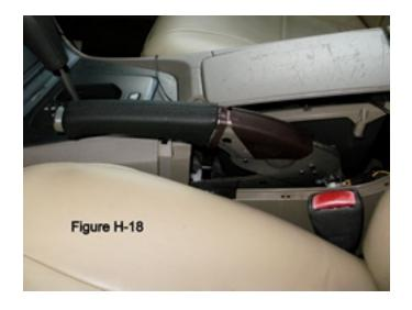
(10) Now, let's put the handbrake boot assembly back in place. Raise the handbrake up to its normal engaged position (to make it easier to get the boot on), then slide the boot over the handbrake handle.
