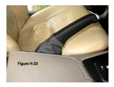
(11) Locate the boot cover alignment pins into their slots, maneuver the cover down into position, and snap it into place. Finally, adjust the leather folds to
