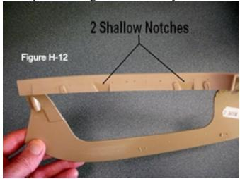
Those two notches in the plastic inner cover will line up (more or less) with the cut-outs along the edge of the leather boot.
