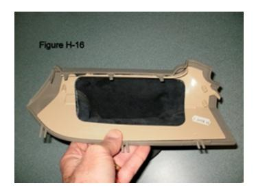
Finally, take the glue gun and run a bead of glue around the edge of the inner cover (where possible) for an extra bit of adhesion. The finished product
