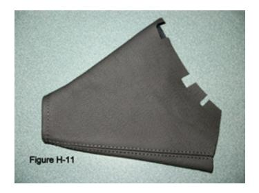
This is a good indicator how to orient the boot on the plastic inner cover. Along the top inside edge of the cover you will see two shallow notches.
