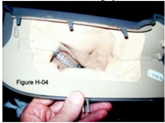
The handbrake boot is sandwiched between the two covers and stapled to the inner cover. Using a small flat-headed screwdriver, separate the inner and outer boot covers by prying the pieces apart at the plastic welds (like small spot welds). They will come apart easily as you break the welds.
