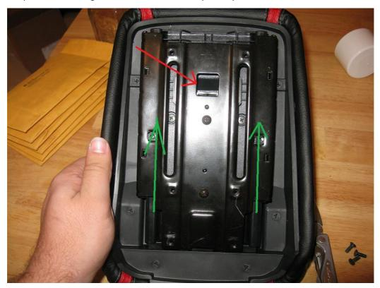
Now you can remove the locking plate and center glide. Basically all the screws come out except the two that hold the metal spring clips:
