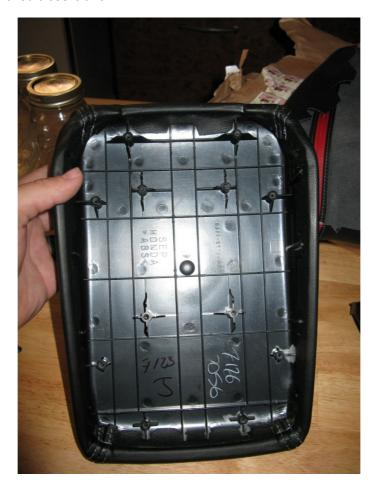
This is where we can start to make a big mess if we aren't careful. First you should give the Wrap a dry fit, just pull the new one over the existing one and pull around it to make sure it will lay smooth:
