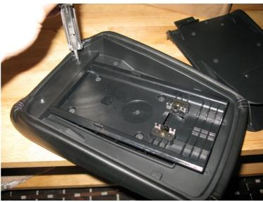
Next the metal glide plate. Then the plastic shroud. Then remount on the center console. I had the metal plate upside down in this picture:
